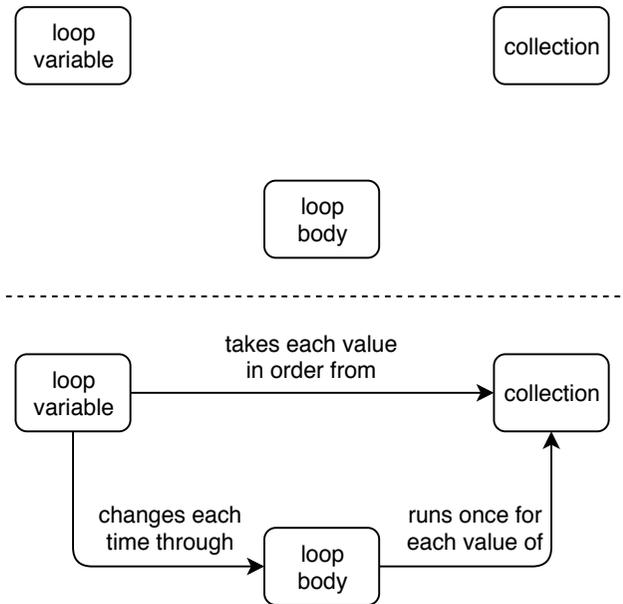
Figure 3.2: Concept Map for a For Loop
