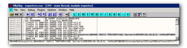
By making use of these credentials, it was possible to make a direct connection to the backend database server to directly access the data.
